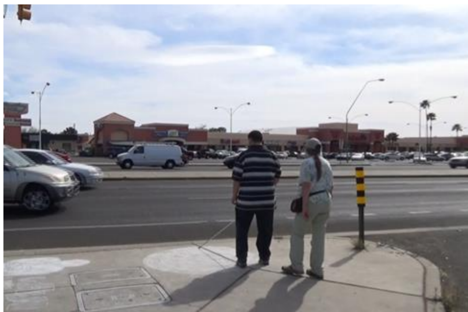
Figure 5-3 Image of a blind pedestrian disoriented on all-paved CTL island
