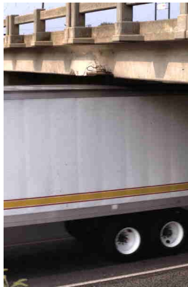
Figure 4.6. Vertical clearance for vehicles at grade separations.
