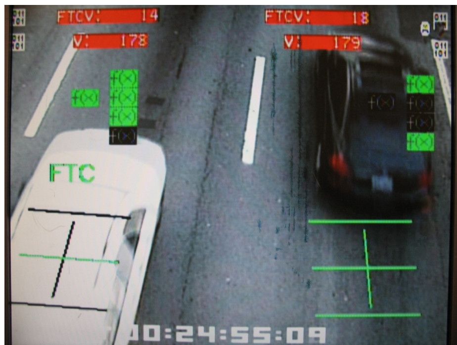
Figure 6. Autoscope view of virtual detectors. Example of speed and traffic volumes by lane.
